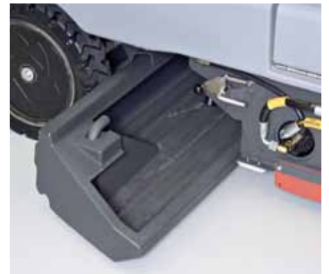
Corrosion resistant hopper slides out easily for maintenance
