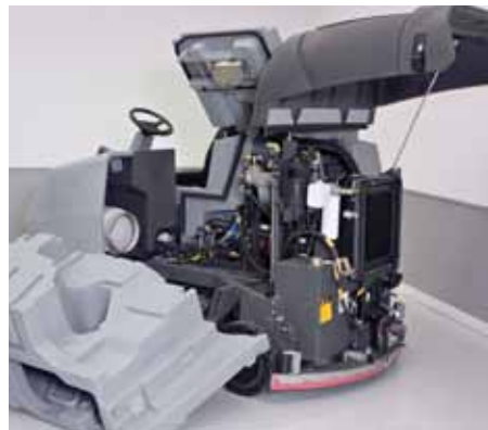
MaxAccess™ design provides 360 degrees access to machine components
